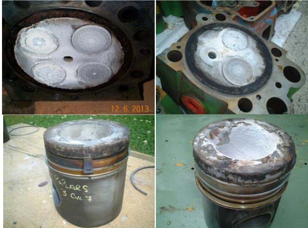
Silica build-up on heads and scrapped pistons of Caterpillar and Jenbacher engines
