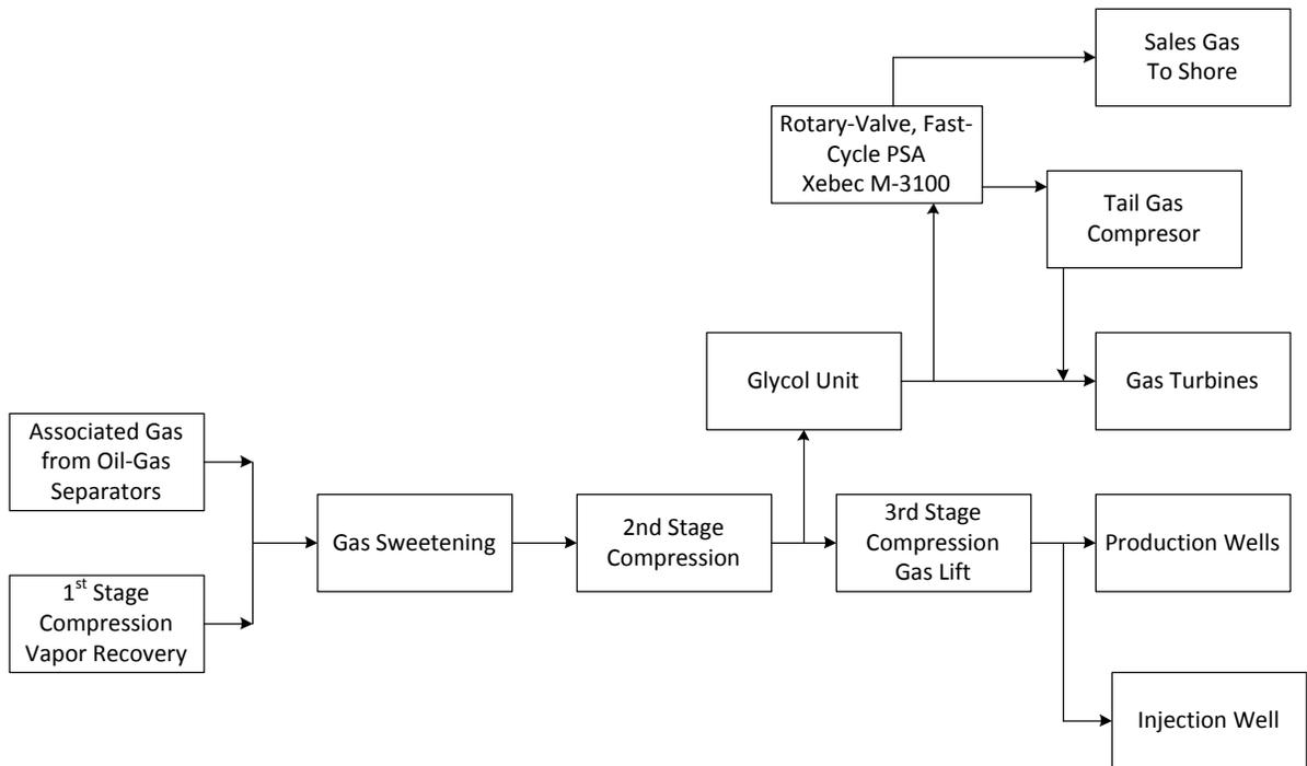
**Figure 5.** Current Platform Gail Gas Block Flow Diagram
