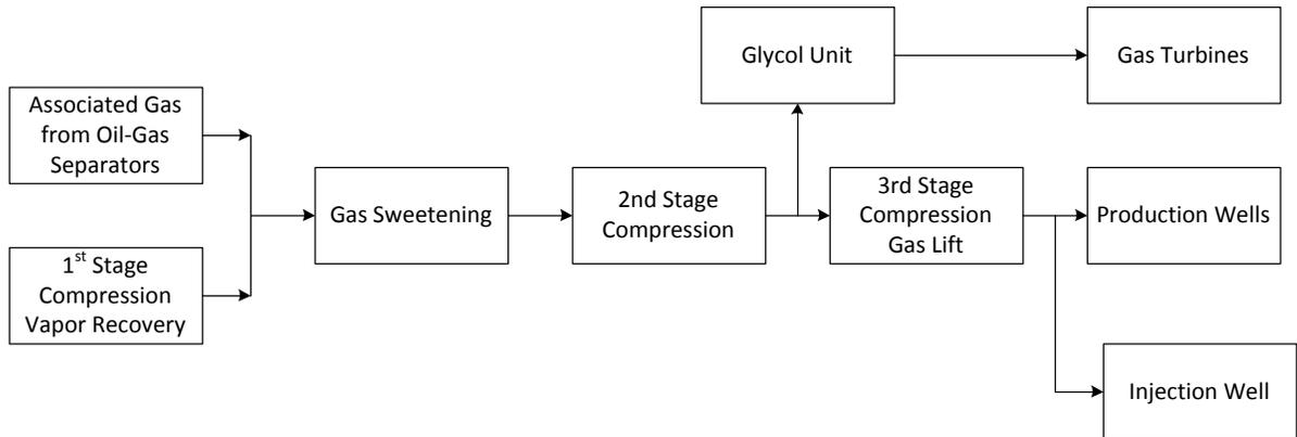
**Figure 1.** Original Platform Gail Gas Block Flow Diagram
