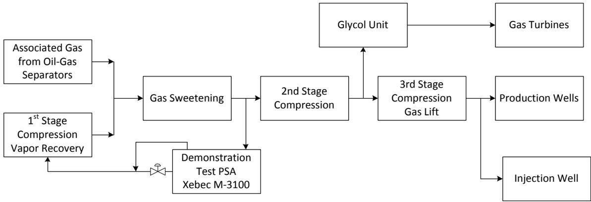
**Figure 4.** PSA Demonstration Test Block Flow Diagram
