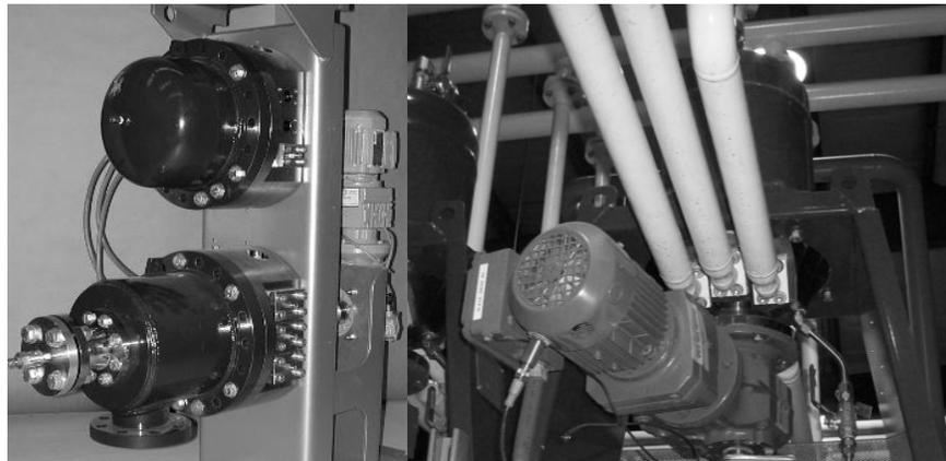
**Figure 2.** Detailed Photographs of Heavies/Lights Xebec Rotary Valves
